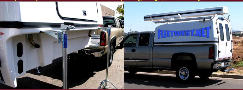
Integrated four corner "no holes" drilled mounting system
